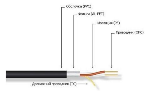
When you are wiring for permanent use, it is recommended that you use cables with at least two twisted pairs in order to be able to use these lines with future versions of the DMX512 protocol. Currently, some manufacturers are already releasing systems using a second twisted pair to transfer information from dimmers to the console. In addition, the additional twisted pair will not interfere if there is an open or short on the main pair.
